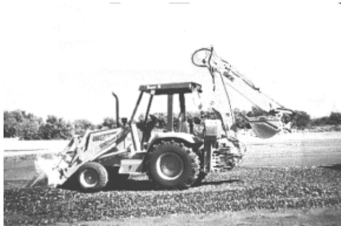
Figure 7-9. Backhoe mounted on farm tractor.
