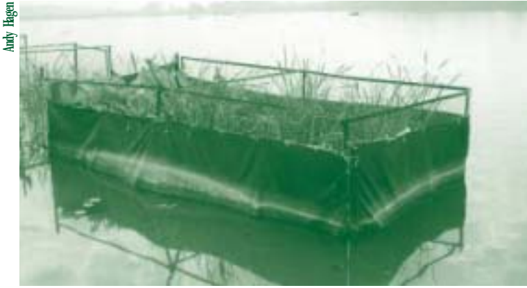
An enclosure with weld-wire fencing T-bars and geotextile.
