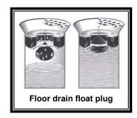
If the plug is not tight enough, pressure can eject it. Therefore, a plug is not recommended for flood depths greater than one foot.
