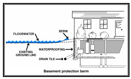
basement walls and the surrounding soil. This will greatly increase the amount of water pressure against the basement walls.
