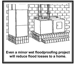
Another approach is to wet floodproof a crawlspace. If your crawlspace has a furnace in it or is used for storage, these items could be moved to the first or second floor. Vents should be placed on the foundation walls to ensure that floodwaters can get into the crawlspace to equalize water pressure.
