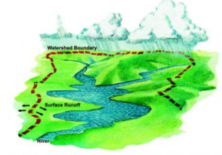
A watershed is an area of land that drains to a common body of water.
