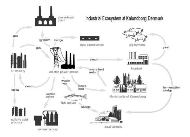
This diagram shows the material and energy flows joining an industrial ecology network in Kalundborg Denmark. Some of the network partners include a gyproc factory, a pharmaceutical firm, a fish farm, a coal-fired electrical power station, a refinery and the municipality of Kalundborg.
