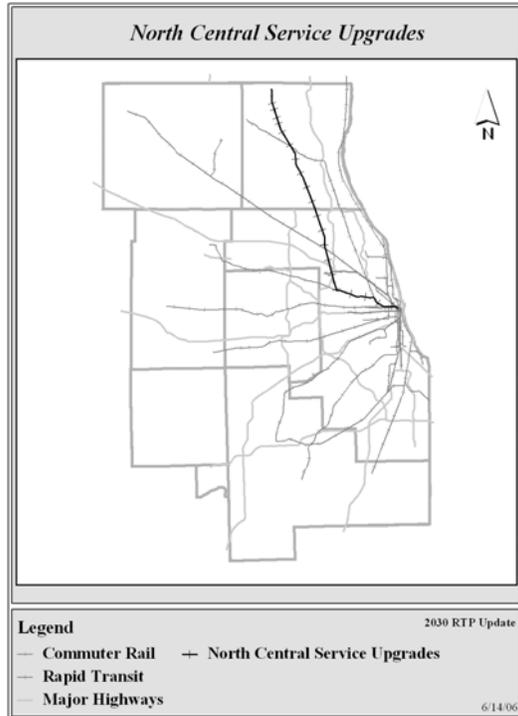
The North Central Service was introduced in August, 1996. The proposal calls for ongoing continuing upgrades to infrastructure and service levels. Phase I improvements to the initial North Central Service Improvements include double-tracking much of the line, new stations, additional parking, and improved operations via the Milwaukee District West Line to Union Station.
