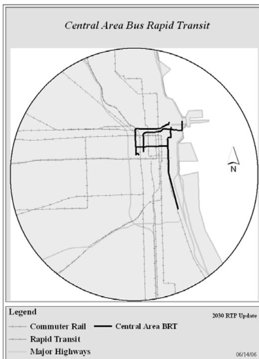
The Central Area Bus Rapid Transit System consists of several components providing improved transit circulation in downtown Chicago. The project would utilize an emerging transit mode called “bus rapid transit,” in which specially designed bus vehicles offer priority transit service on arterial streets or dedicated rights-of-way with rapid boarding and alighting.
