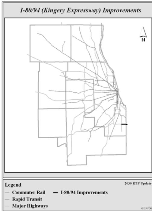
I-80/I-94 provides a link between northern Illinois and the northern tier of the United States. It is a critical trucking route and serves large numbers of external trips. The proposal is to provide additional capacity on I-80/94 from I-294 to US 41, plus a major new collector/distributor system servicing the I-294/IL 394 interchange.
