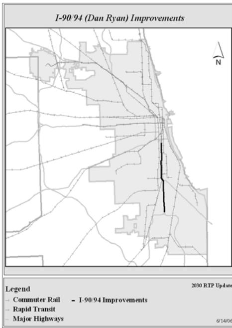
This project consists primarily of reconstructing the existing roadway and reconfiguring access to improve safety. Modified access and auxiliary lanes will be included in the project to reduce weaving maneuvers. Through-access on I-90 to the Chicago Skyway Toll Bridge will be enhanced with a flyover to the express lanes north of 63<sup>rd</sup> Street.
