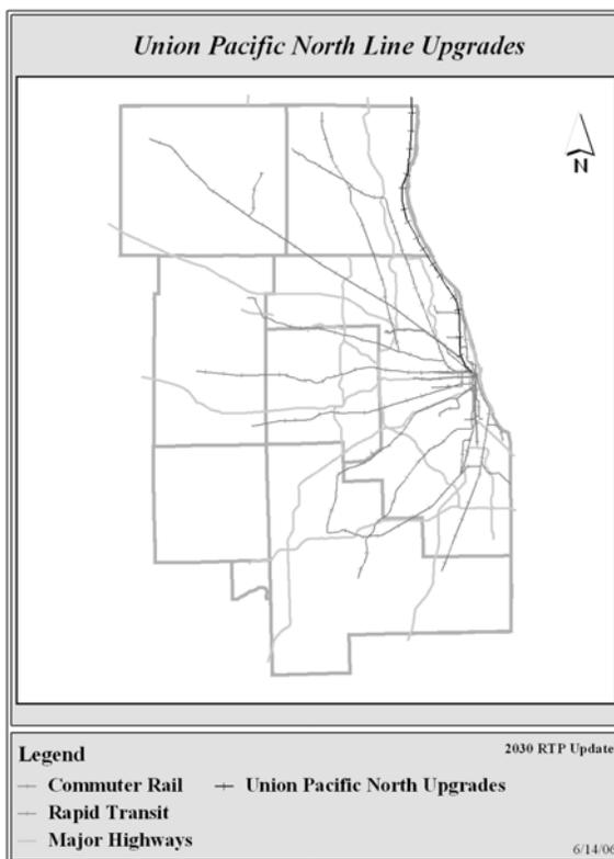
The Union Pacific North Line serves Chicago, northern Cook and Lake Counties. The proposal is to upgrade the existing signal system and install additional crossovers between downtown Chicago and the outer terminal in order to increase the operating capacity of the UP-N Line.
