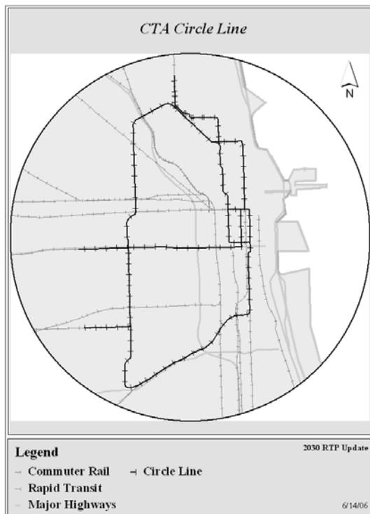
The Circle Line is composed of new strategic links to Chicago's rapid transit system that will allow more direct connections between rapid transit and commuter rail lines serving the region's core. These new links are located in a ring about two to three miles from the Chicago Central
