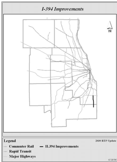
IL394 connects southeastern Will County to the rest of the region. The highway is also expected to be a key access route to the proposed South Suburban Airport. The initial proposal is to add lanes from I-80/94 to south of the proposed IL394/I-57 connector road and to convert from the existing high-type arterial to freeway design from US30 to south of the proposed IL394/I-57 connector road. From the connector road to IL1, the road would remain a controlled-access arterial road.
