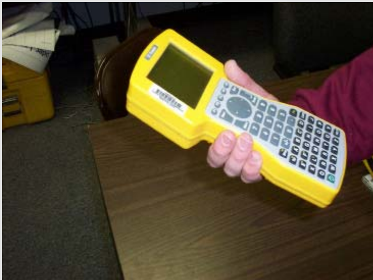
The above data logger is used as the interface device for a GIS backpack unit.
