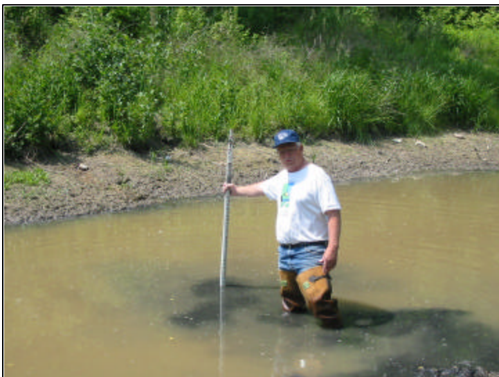
Don in the wetland forebay with the measuring rod. There was 0.5 feet of organic silt on the bottom and 1.5 feet of water in the forebay.
