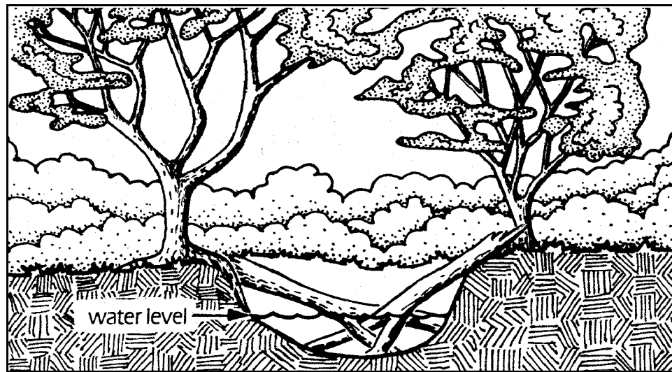
Exhibit 5.4b: Illustration of a Condition 2 Logjam (Source: American Fisheries Society Obstruction Removal Guidelines)
