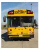
pants in the Illinois Clean School Bus Program. Illinois EPA provided a grant to the district to retrofit 93 school buses with diesel oxidation catalysts that reduce emissions of particulate matter. In addition, the entire bus fleet is using biodiesel fuel, a blend of 20 percent soy oil mixed
