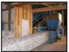
Knowing the type and volume of material requiring baling, along with any space limitations, will help in determining whether a horizontal baler or a vertical baler would be the appropriate choice for a given application. Due to the cost and the need to handle varied materials, many smaller facilities rely upon a single large, single-ram horizontal baler.
