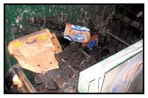
the single-stream material back into the dual streams of fiber and containers. Sometimes multiple screens are used to subsequently separate OCC from ONP and mixed paper.
