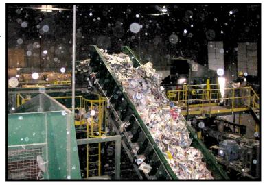
where they pass through an optical sort unit that uses sensor-controlled air jets to remove all plastic bottles. Bottles are not sorted by resin type. At the end of the line a final sort for UBCs is done with an eddy current separator.
