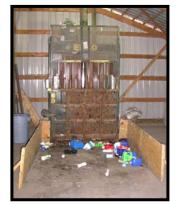
Some MRFs have employed dedicated balers with hoppers for each baleable container commodity. However this system suffers from lack of sufficient storage in the hoppers, extra maintenance associated with the balers, and low bale densities associated with the smaller balers used.
