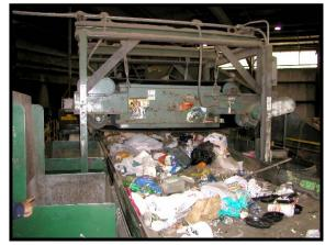
determined from various spectrographic or electromagnetic signatures. The sensors then trigger mechanical or pneumatic devices to remove the identified items from the conveyor. These systems are quite expensive and are typically used only in the largest MRFs.
