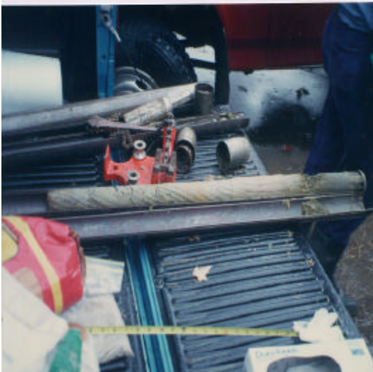
Soil from a boring is ready for field screening.
