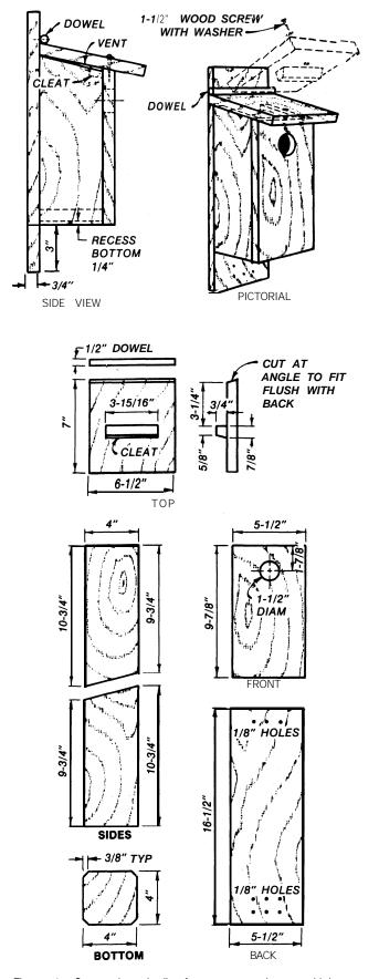
Figure 1. Construction details for a top-opening songbird nest box.
