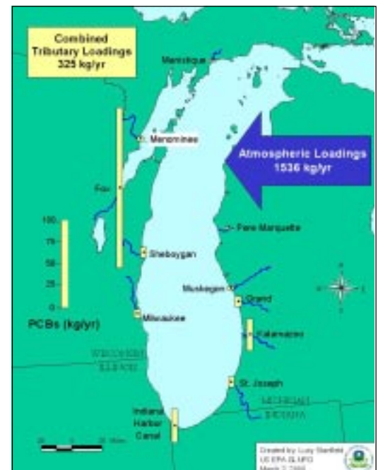
A large portion of the PCBs loadings to Lake Michigan are coming from the atmosphere.
